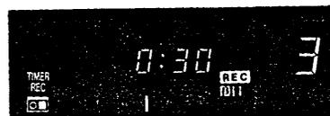
When the recording starts, the time indication decreases minute by minute to 0:00 and the recorder turns off automatically.
